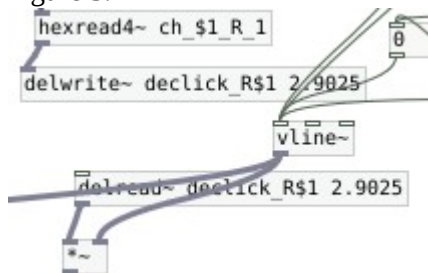
Figure 2. The vline~ object is used to attenuate delayed audio while changes happen to the source array or read point.
