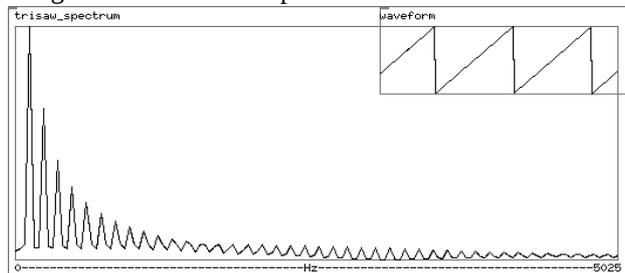
**Figure 2.** Spectrum and waveform at symmetry setting 1 (ramp waveform).
