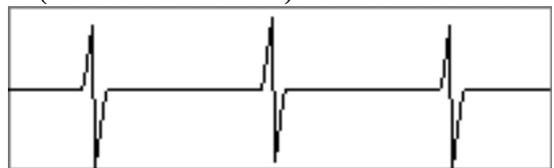
Figure 10. With the same sawtooth input, breakpoint = -0.75, stretch factor = -1.
