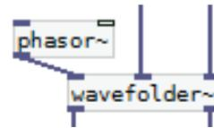
**Figure 1.** The wavefolder~ object generates variable asymmetry sawtooth/triangle waves from a phasor~ (ramp) input.
