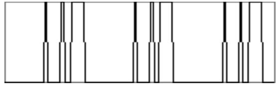
Figure 8. An example of the pulse-width modulated output from `wavfolder~`.
