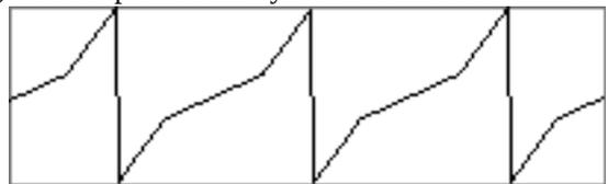
Figure 9. Stretched sawtooth waveform at breakpoint = 0 (middle of absolute value) and stretch factor at -0.5.
