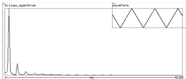
**Figure 5.** Spectrum and waveform at symmetry setting 0 (triangle waveform).
