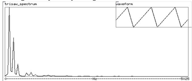
**Figure 4.** Spectrum and waveform at symmetry setting 0.5.
